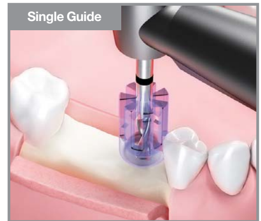
Single Guide enables correct measurement through close attachment
